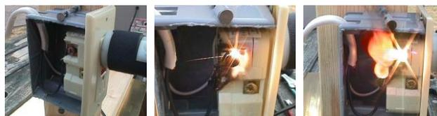
Fig. 8 Ground fault receptacle, with glowing contact, on fire
