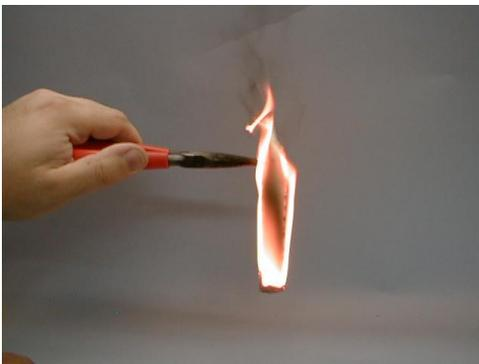
Fig. 14 Flammability test of glass electrical tape
